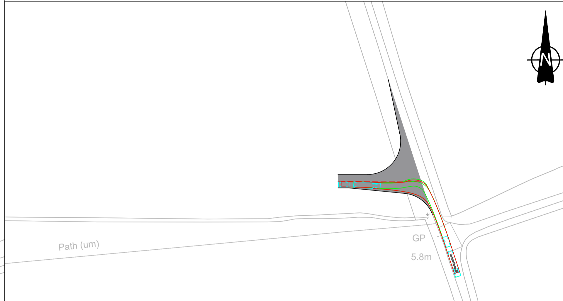
INSET B: TRACTOR & HAY WAGON MANOEUVRE HEADING NORTH, LEFT TURN INTO ACCESS - SCALE 1:1000
