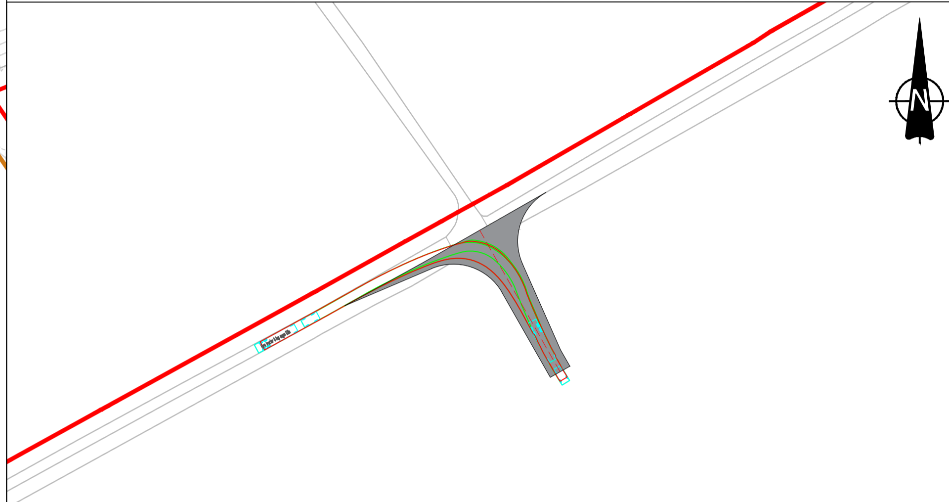
INSET B: FARM TRACTOR AND HAY WAGON MANOEUVRE HEADING EAST ON INGS LANE RIGHT TURN INTO ACCESS- SCALE 1:1000
